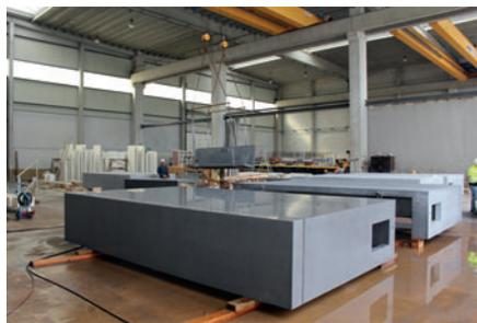
Decomo SA producers precast elements in architectural concrete
