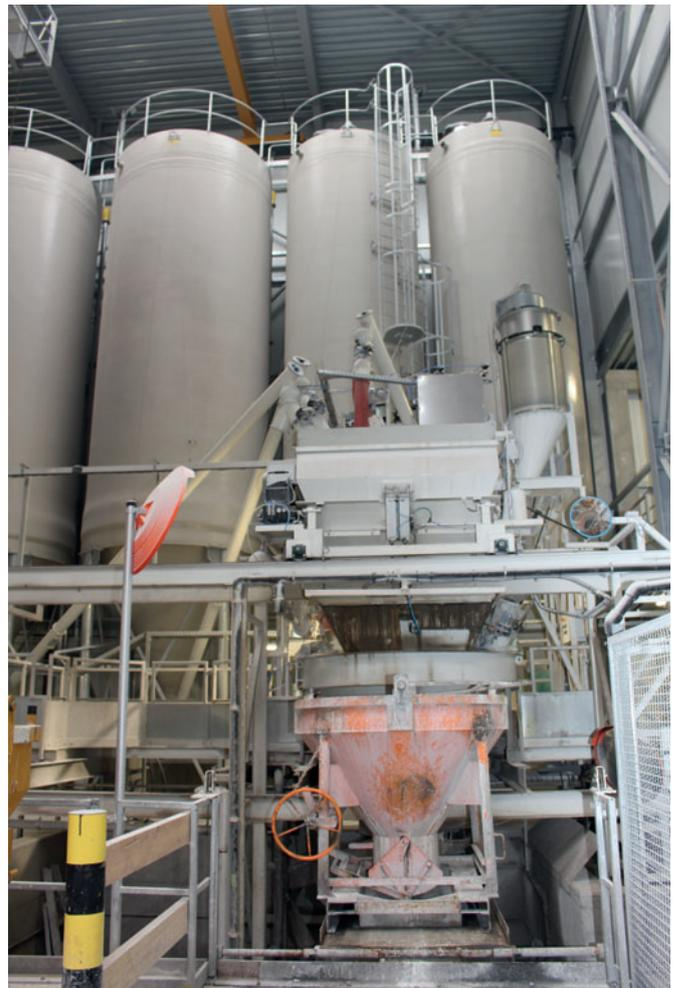
*The mixer empties directly into a concrete bucket that is delivered empty to the concrete mixer by means of a scissor lift mounted on a mobile trolley.*
