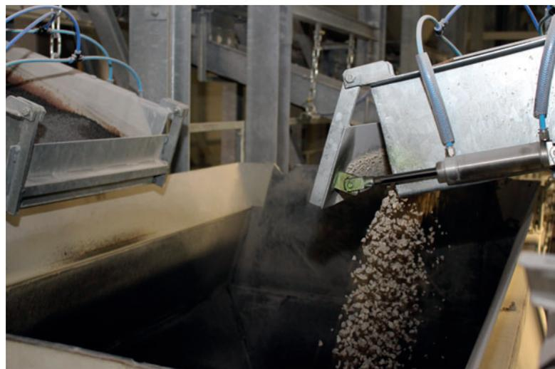
Precise dosing of aggregates in the mobile scale is carried out with vibrating chutes and shut off dampers.
