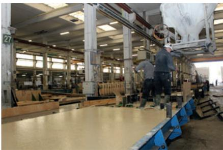
View inside the production hall with the new Construx tilting tables
