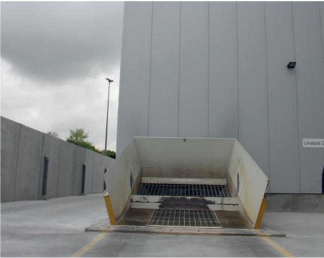
Charging of the aggregate silos is initially carried out from the exterior using a truck charging hopper.
