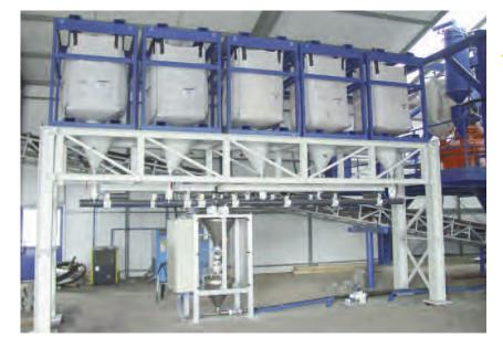
COM 70-1 Granular Metering System for 5 colors in 2 mixers with one weigh hopper, one pressure vessel and one diverter valve
