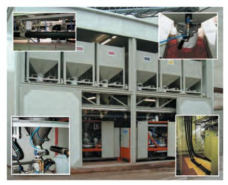
Combined Granular Metering System with two COM 70-2 for 6 colors in 4 mixers with 2 weigh hoppers and 4 pressure vessels. System is equipped with 6 change containers for low profile design
