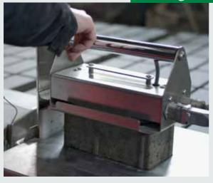
The QAVER® is a testing device, developed to measure the quality of the freshly produced concrete product. The following properties can be determined by the QAVER®:
